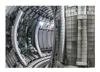
JET is the largest tokamak in the world. In operation since 1983, JET was explicitly designed to study plasma. Today, its primary task is to prepare for the construction and operation of ITER, acting as a test bed for ITER technologies and plasma operating scenarios.
